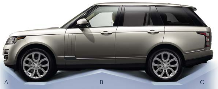
Obstacle Clearance Off-road height 296.1mm Standard ride height 221.1mm
