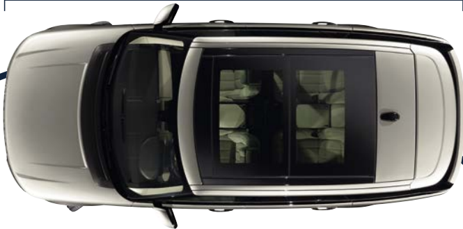
Turning Circle Kerb-to-kerb 12.1m (Long Wheelbase 13.0m) Wall-to-wall 12.5m (Long Wheelbase 13.4m) Turns lock-to-lock 3.03
