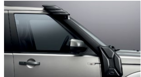
Raised Air Intake
