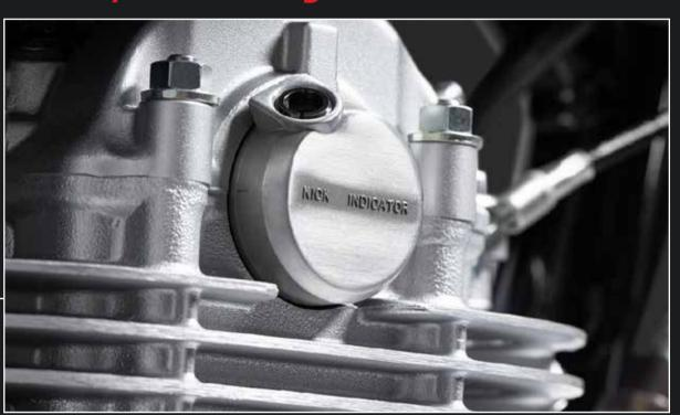
To underline our commitment to originality the SR400 is equipped with a kick starter as the only means of getting the engine running. Starting is made easier by the decompressor lever on the handlebars and a piston position indicator on the side of the cylinder head, as well as the new fuel injection system.
