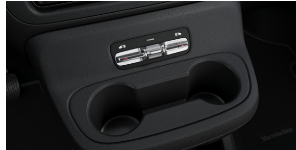
Electrical operation of sliding doors
