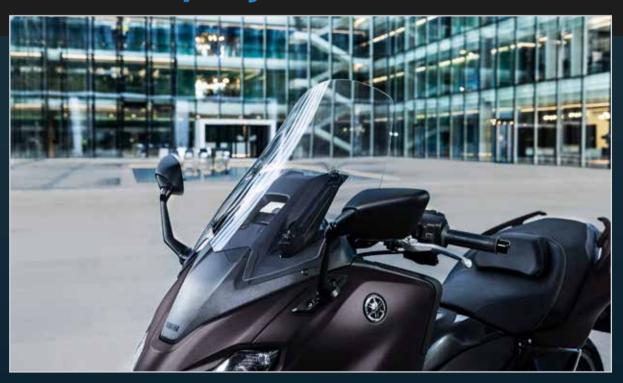
The adjustable windscreen features a centre air intake duct that contributes towards the increased level of comfort by reducing pressure on your upper body, especially at higher speeds. This new design also ensures better acoustics when you're using a smartphone linked to the 7- inch TFT full-colour display, and the TMAX Tech MAX screen can be adjusted electrically using a handlebar mounted switch.
