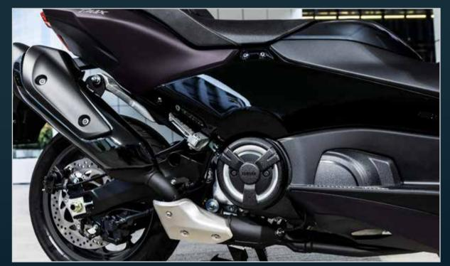
The powerful 560cc EURO5 engine features a unique and compact design that uses a 360 degree crank with a horizontally opposed reciprocating piston balancer for extremely sporty performance together with a high-efficiency CVT drive system for outstandingly smooth running. And to heighten your riding excitement the carefully designed intake and exhaust systems produce a deep and pure 'tuned' sound that is distinctively TMAX Tech MAX!
