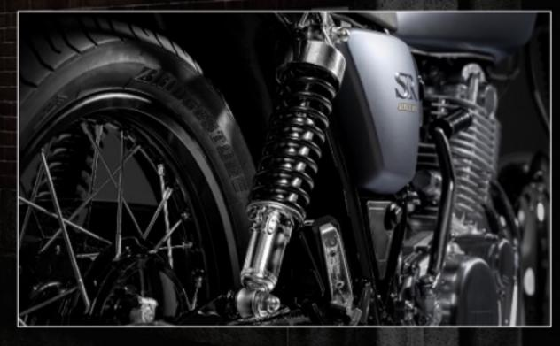
The SR400 is equipped with traditional suspension that gives a plush and comfortable ride, with the front forks giving 150 mm travel and the twin shocks at the rear giving 110 mm wheel movement. And with its slim fuel tank, raised handlebars and long dual seat, the SR400 benefits from a natural and relaxed riding position
