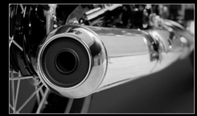
While remaining true to the 400 S.R's original design and concept, we have also taken the opportunity to make a number of technical improvements such as the fitment of fuel injection and transistor ignition for good economy and easy starting. And for reduced emissions the chrome exhaust system features a 3-way catalyzer.
