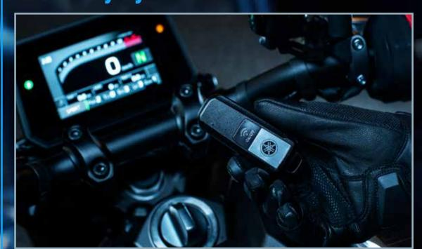
Taking the next leap in technological advancement, the MT-09 SP becomes the first Hyper Naked to feature Yamaha's Smart Key System. The engine is started by pressing and turning the newly designed switch, provided that the smart key is within a specified range such as in your pocket. The all-new switch also features a lock and unlock option for the fuel tank cap, further simplifying the riding experience.
