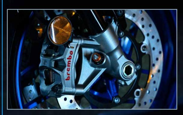
New Brembo monoblock Stylema@ calipers refine braking performance with the very latest technology from the famous Italian firm. The calipers feature a slimmer piston and brake pad area, compared to conventional calipers, as well as being lighter, more rigid and offering enhanced control in braking input. In addition, larger diameter pistons are adopted for increased braking forces allowing you to experience the next level in braking performance.
