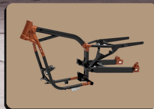
FRAME WITHOUT WELDING POINT
