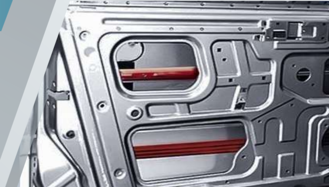
Anti-Collision Steel Beam in Door
