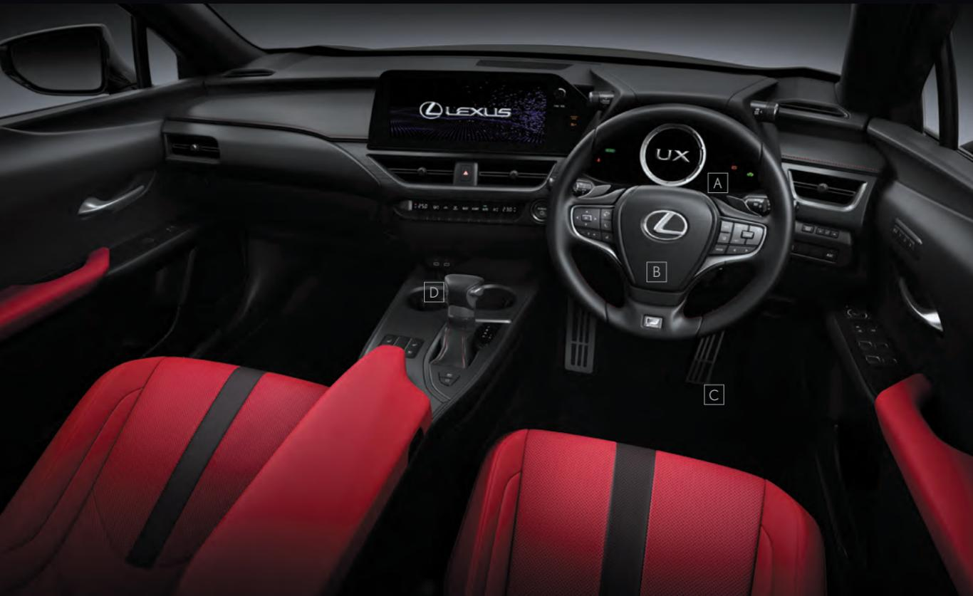
A\_Meters & multi-information display / B\_Steering wheel / C\_Aluminum pedals / D\_Shift lever knob
