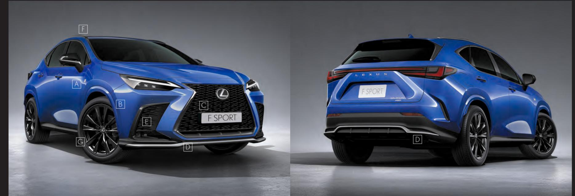
A\_F SPORT emblem / B\_Fender arch moldings / C\_Grille / D\_Lower bumper spoiler / E\_Garnish / F\_Roof rails / G\_Exclusive 20-inch aluminum wheels
