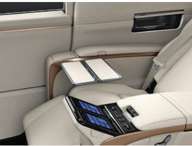
ARMREST TABLE AND STORAGE Each chair's outside armrest contains a stowable table that can serve as a stable foundation for a tablet, notebook, or laptop computer. While deployed, the table can rotate, allowing for easy reach into the refrigerator. The inside armrest features a two-way opening console lid that covers a useful storage area.
