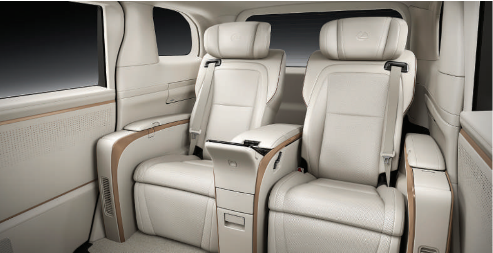
SOFT SURFACE LAYER Two types of vibration-absorbing materials – low-resilience foam (high viscoelasticity traits) and urethane (high sitting pressure dispersion quality) – encompass the body to provide proper support, reducing vibrations transmitted from outside the vehicle. FIXED HEADREST A large headrest features a high-back design and concave center cushion to accommodate a wide range of head sizes and shapes, as well as body postures.
