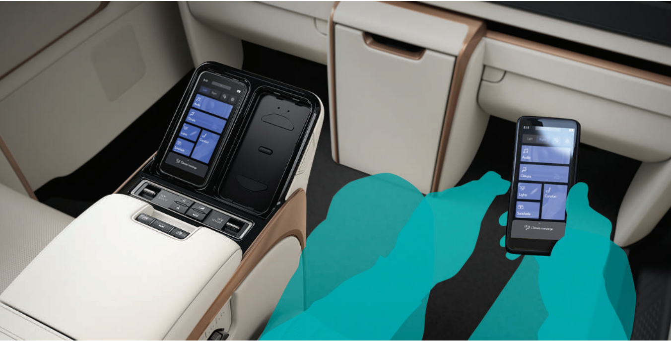
MULTI-OPERATION PANEL Located atop the center console's front edge, the panel consists of two independent remote controllers that command rear seat functions, as well as Lexus Climate Concierge, audio, and ambient illumination settings. A warning buzzer sounds when the controllers leave the interior's immediate vicinity. LEXUS CLIMATE CONCIERGE A one-stop, integrated control of the rear area's comfort equipment, including seat reclining, air conditioning, ambient illumination, and shade functions. Passengers can select one of five pre-set modes – Dream, Relax, Focus, Energise, My Original – on the multi-operational panel controllers that best reflect their desired environment. The system automatically adjusts the comfort equipment's settings based on temperature readings taken from an infrared matrix sensor located at the partition's top center. The sensor detects the temperatures of the area's surfaces (windows, trim, ceiling, etc.) and estimates the warmth of four body areas (face, chest, upper leg, lower leg) during its adjustment and application of air conditioning and seat heaters/ventilation.
