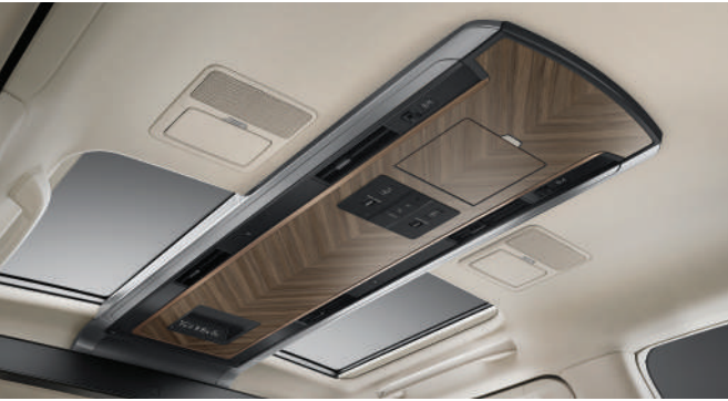
OVERHEAD CONTROLS A sleek control panel sits above and center of the rear seats. Settings for window shades, roof sunshade, ambient illumination, and air conditioning can be adjusted via the control panel. Dual LED-illuminated vanity mirrors can be tilted to an increased 140 degrees for improved visibility when checking one's neck area or tying a tie.
