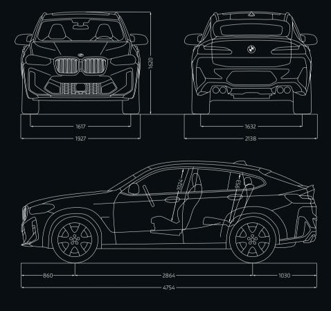
The dimensions in the technical drawing are in millimetres and may vary depending on the model and equipment.
