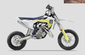
Tapered NEKEN handlebar Die-cast aluminium swingarm Chromium-molybdenum-steel frame Adjustable WP XACT fork & PDS shock
