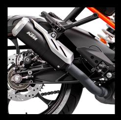
Taking its design cues from the MotoGP™ RC16, the exhaust of the KTM RC 390 boasts stainless steel headers with an aluminum muffler, which not only look the part but give the KTM RC 390 a distinct, throaty rumble as it charges through the gears and onto the redline.
