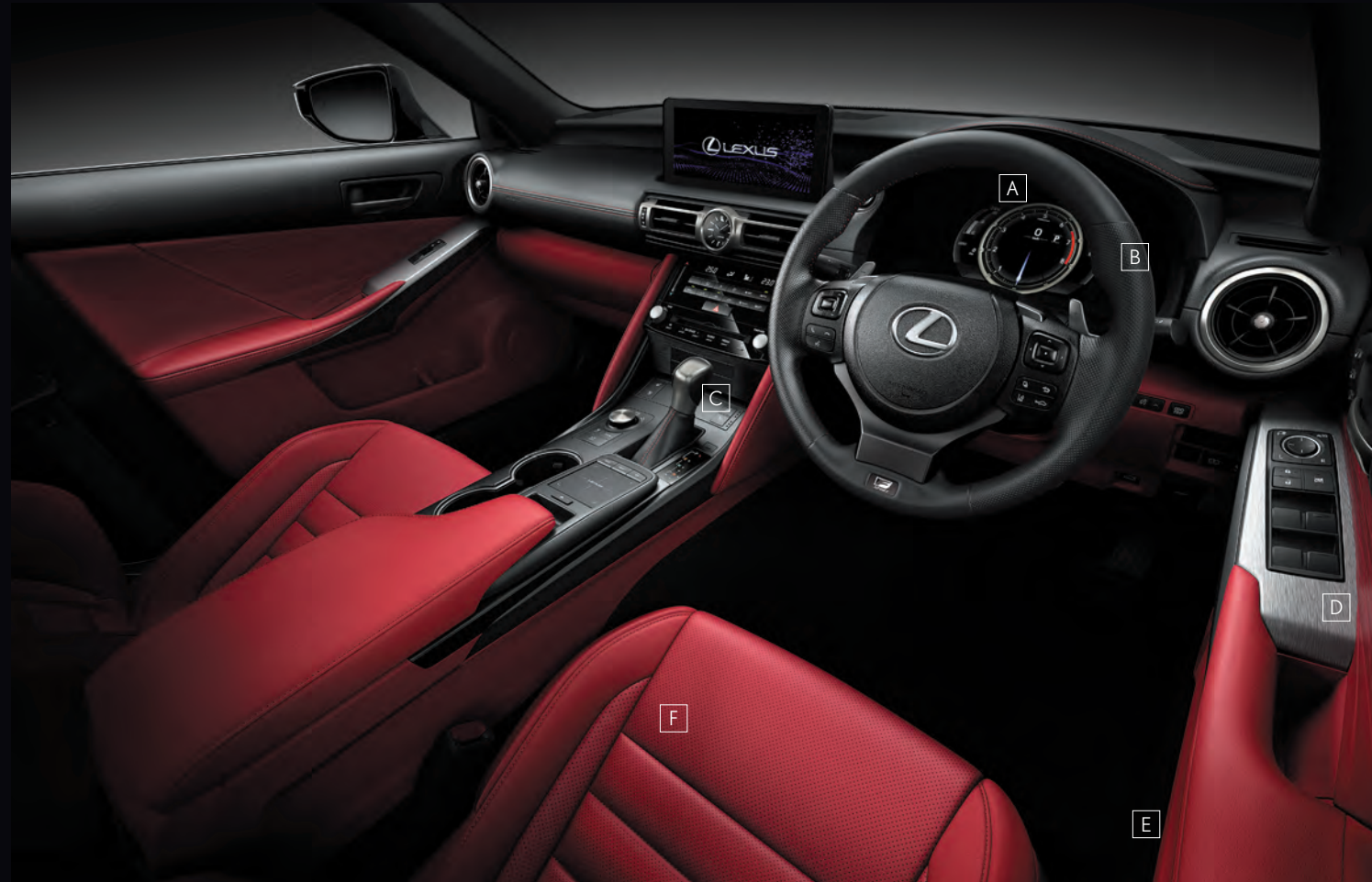
A_Single dial meter / B_Steering wheel / C_Shift lever knob / D_Trim / E_Scuff plates / F_Front seats
