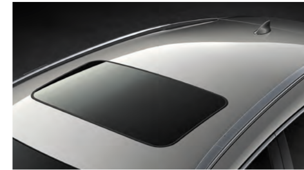
Moon roof* On the moon roof, the inner glass unit slides open, enabling a more expansive opening when the roof is fully open.
